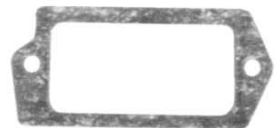
Outer gasket for muffler to manifold
