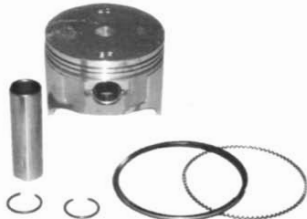
Piston & ring sets available for 350cc engine
